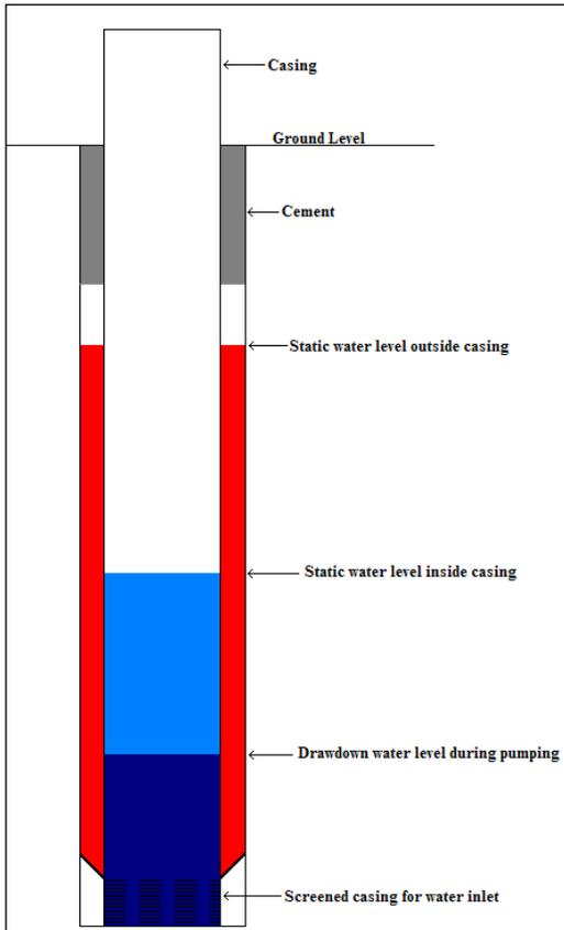
The casing is the most important part of a water well system. Without it, your well collapses and will have to be drilled again. For years, the drillers in this area have struggled with casing collapse. The column on the outside of the casing fills up with seep water, while the water inside the casing pushes back out. When the water level drops during pumping, the water on the outside pushes in on the casing. This is even worse during drought periods. If the pressure on the casing is
